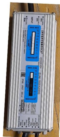
Figure 4: h=368 LED DRIVER - Thermal Test
